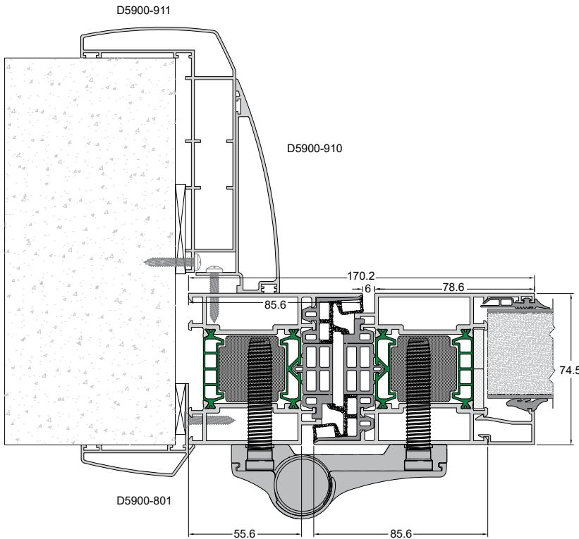
D5900 is designed to cover the finishing of vertical and horizontal sections of the wall. Suitable for interior and exterior use of vertical wall sections in which the thickness of the frame is not sufficient to cover the transverse and longitudinal sections of masonry. With the wall section cover, the architectural aluminum system is in line with the rest of the structure, allowing a perfect and harmonious effect on the overall appearance of the construction, masonry-door-window.
