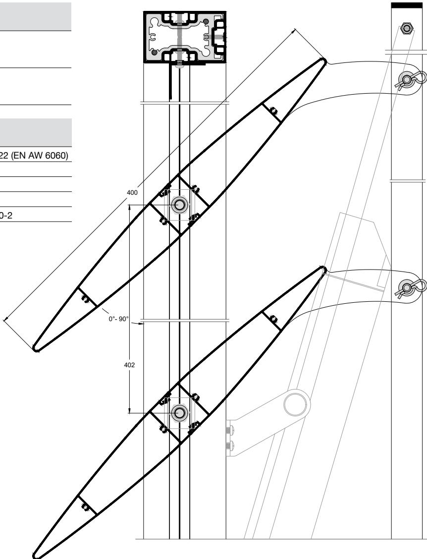
Elliptical design louver with adjustable incline
