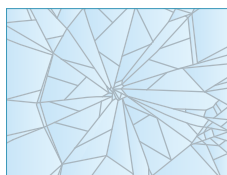
Laminated Glass TRIPLEx glass with PVB membrane
