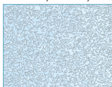
Toughened Glass Thermally Toughened glass
