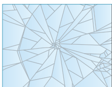
Laminated Glass TRIPLEX glass with PVB membrane
