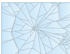
Laminated Glass TRIPLEX glass with PVB membrane
